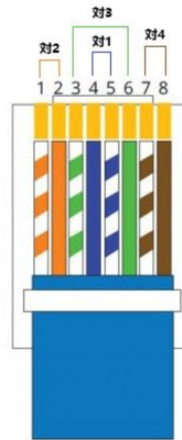
RJ45 Pinout T-568B
